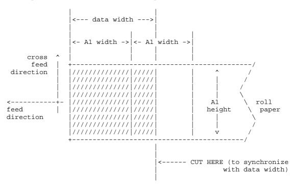
Example 2: "Auto-Cut", a device cutting the roll paper at multiples of fixed-size media width
